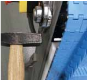
3 Gently tap its head into retaining position
